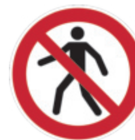
No pedestrians allowed (ASR A1.3)
